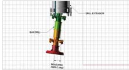
Fig.5 – Angle between Drill Extension and BHA DR
