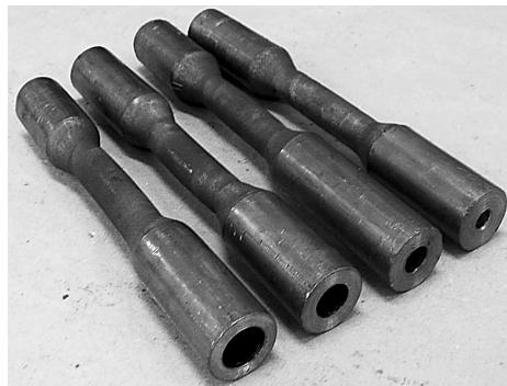
FIGURE 3. Hollowed shafts formed in the CWR process of flat wedges
