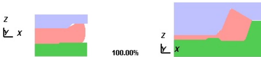
Figure 12. Net shape forging using centered lower die (case--3)
