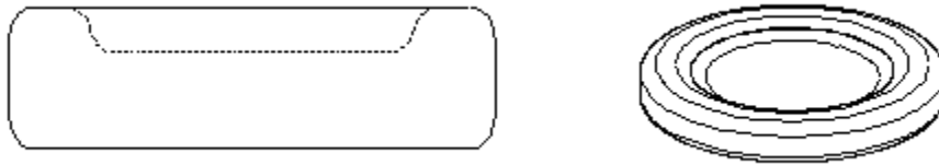
Figure 8. Preform obtained by volume mapping approach
