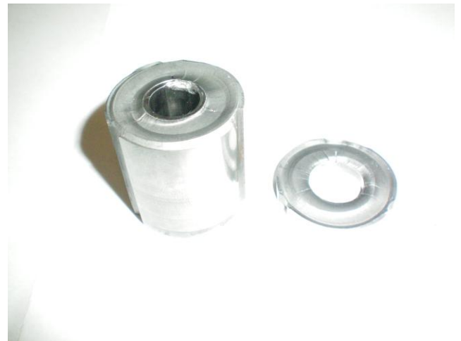
Figure 3: Baseline – Typical Die Failure
