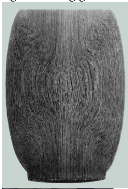
FIGURE 4. Deformed fibers in step height
