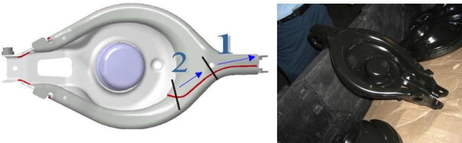
Welded assembly of sheet metal formed parts in the automotive industry
