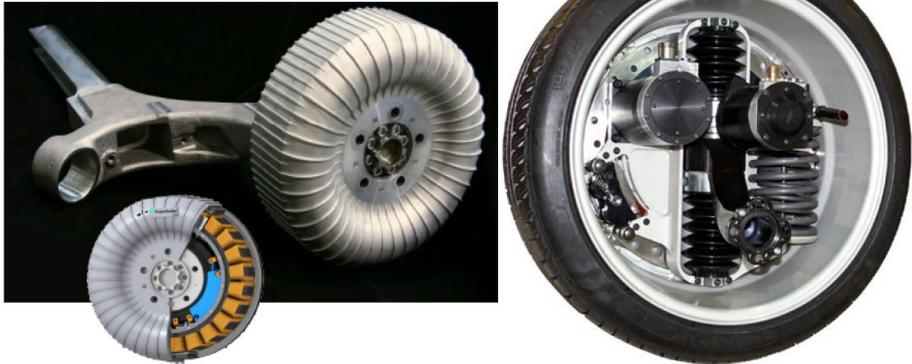
Left: torsion beam axle with electric engine ; right: Active Wheel from Michelin
