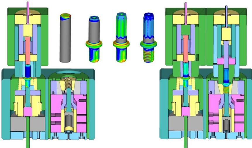
Simulation model of a complex tool assembly of a tool concept for thread embossing
