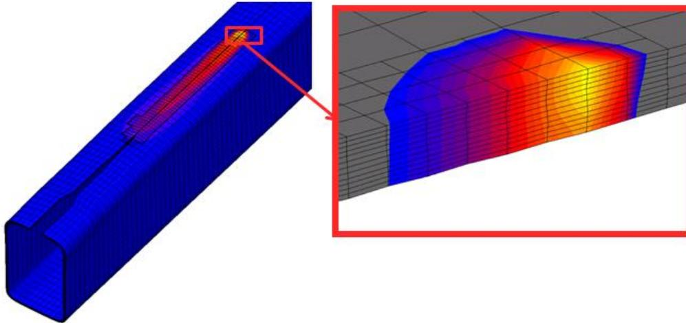
**Figure 5. Automatic adaptive mesh refinement as heat source moves along the weld-path**
