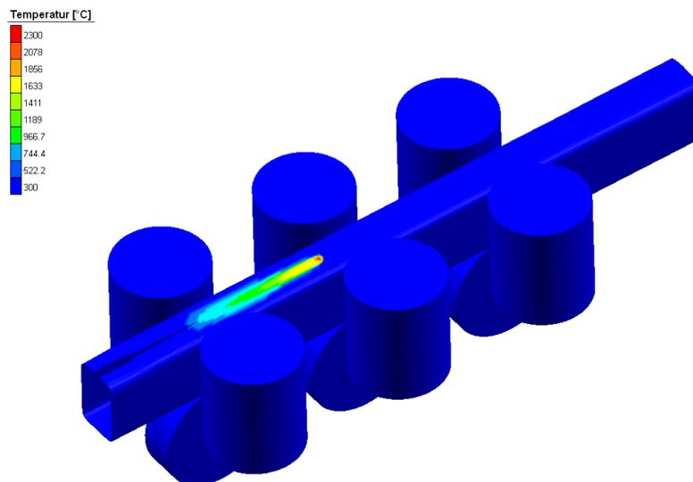
**Figure 6. Model setup, including side-rollers that push the profile shut**
