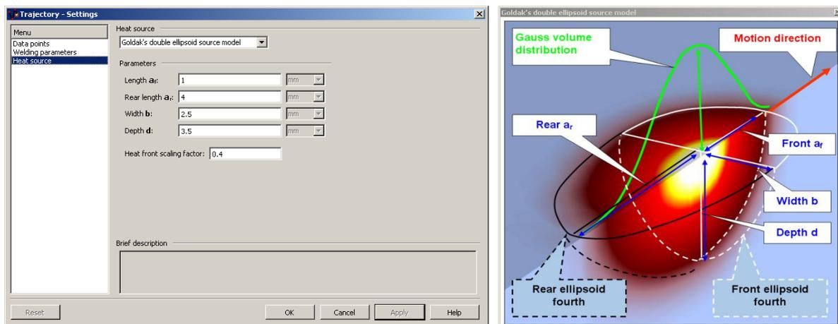
Figure 4.Definition of the heat-source of the welding process
