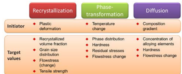
Figure 2: Most important physical effects for the microstructure during forming and heat treatment
