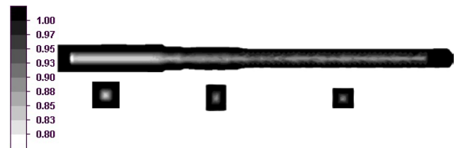
Figure 6: Relative density after the cogging process, cross section lengthwise (above) and crosswise (below)
