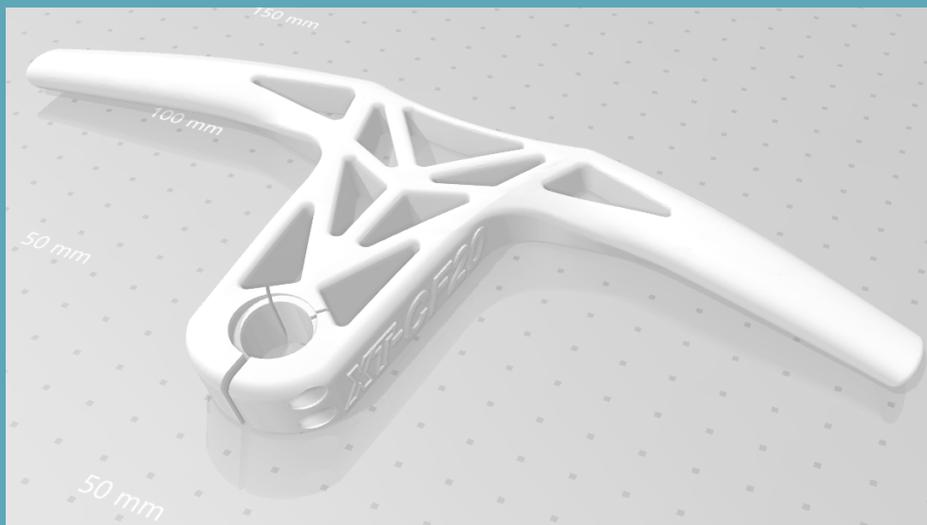
Figure 3: 3D printed polymer bike handle
