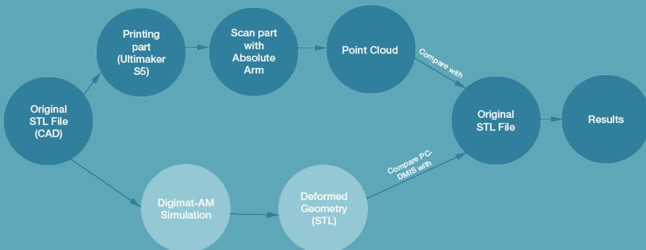
Figure 4: Digital continuity chain for the 3D printed bike handle case
