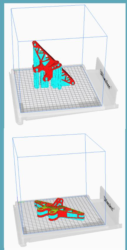
Figure 1: Multivariable analysis of a 3D Printed Polymer Bracket with upright and flat printing orientations
