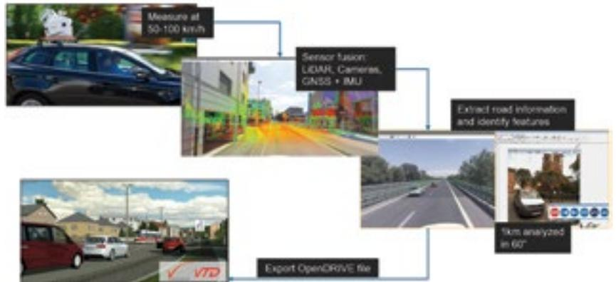
**Figure 5. Creating Virtual 3D Environment in VTD from Metrology Road Measurements**
