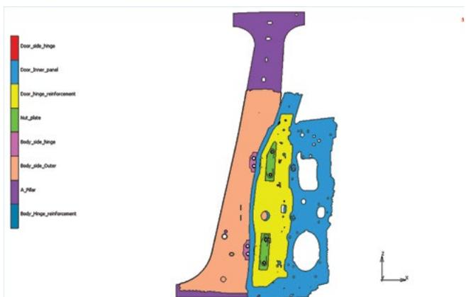
Figure 3: HM table for Door Sag and resultant template
