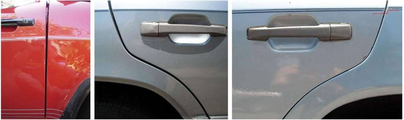
**Figure 1: Examples of door sag in automobiles**
