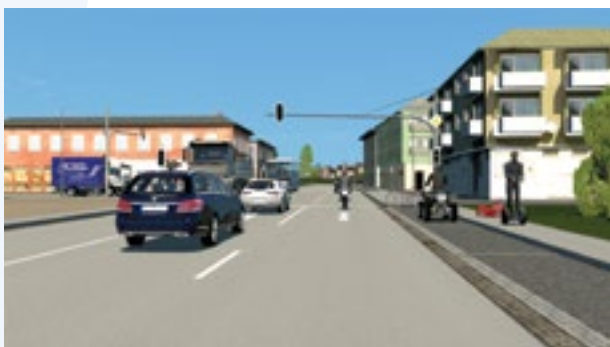
Figure 1. A typical scenario to test an autonomous driving system using VTD
