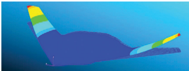
Figure 3: Non-linear UAV shape prediction of wing deflection displayed in the Toolkit
