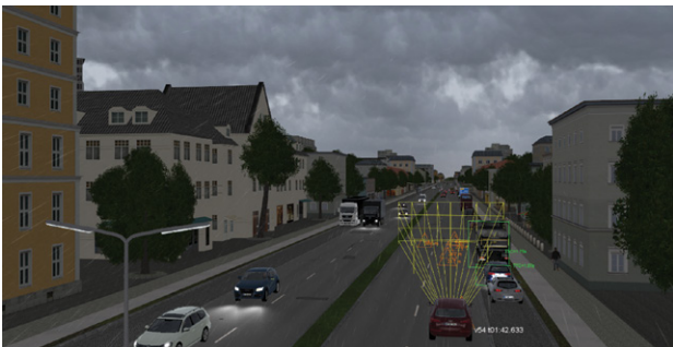
Figure 1. Virtual Sensor Models in VIREs VTD Environment
