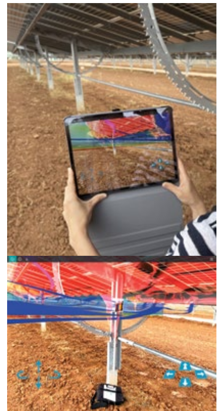
Figure 5: Cradle CFD's Digital Twin flow prediction at Hexagon's Archidona Solar Farm in Xalt Augmented Reality iPad viewer
