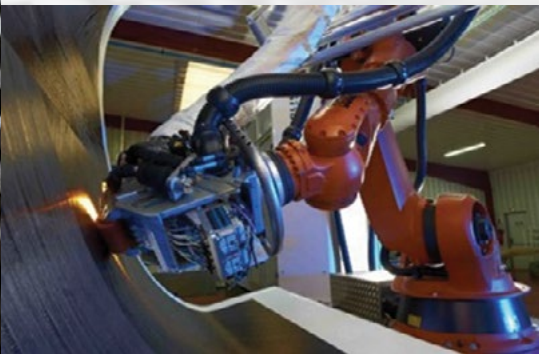
Figure 1: Automated Fiber Placement robotic system (Coriolis Composites)
