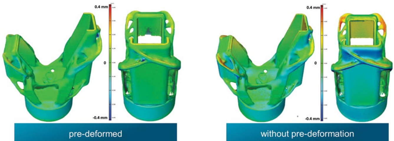
On the left, the measurement result of the preformed part can be seen, which is significantly lower than that of the right, unadjusted part. Thus, Simufact Additive could achieve a significant improvement of the part quality here. Source: SLM Solutions
