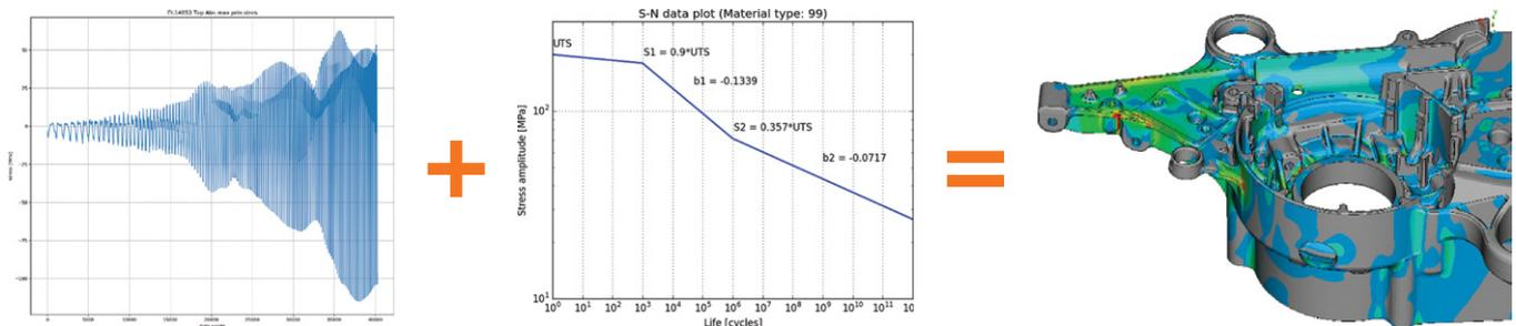
Figure 4 Nastran Embedded Fatigue Process: Structural Analysis Results + S-N Data Plot = Fatigue outputs such as stress, Damage, Life
