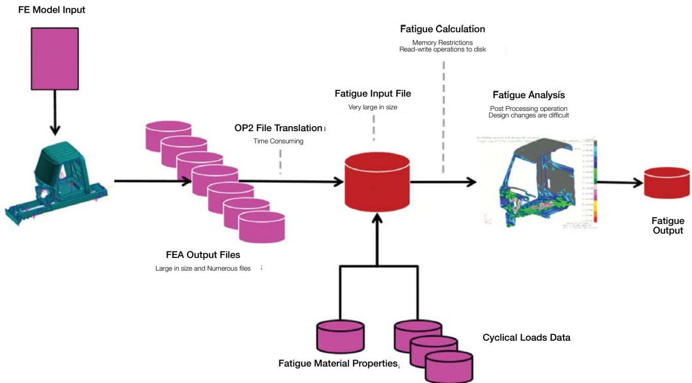
Figure 2 Traditional Fatigue Analysis Workflow
