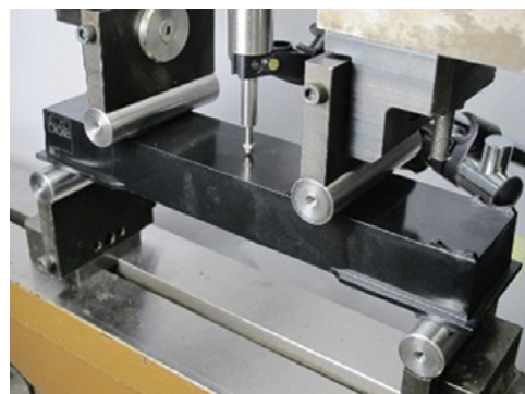
Figure 2-b: Four points bending test set-up (4PB).
