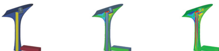
Picture 4 and 5 and 6: Impact analysis in Marc software. The heel of the shoe is made of an exterior, connection and spine which is impacted by a blunt object.
