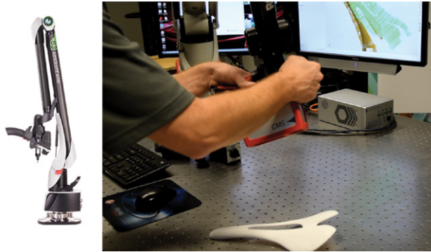
Figure 11: Final inspection of the 3D printed polymer seat part Hexagon Absolute Arm
