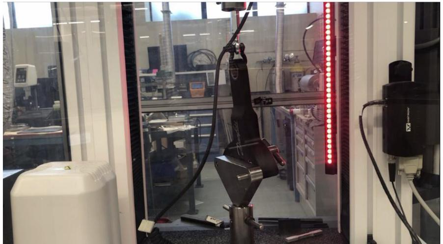
Danfoss' lifting tool has been physically tested to failure on an Instron machine. The simulation results of the Onyx-only part are in good agreement with the experiments: the failure location (close to the hole where the loading is applied) is accurately predicted, and the maximum force that can be applied underestimates the physical test by 25%.
