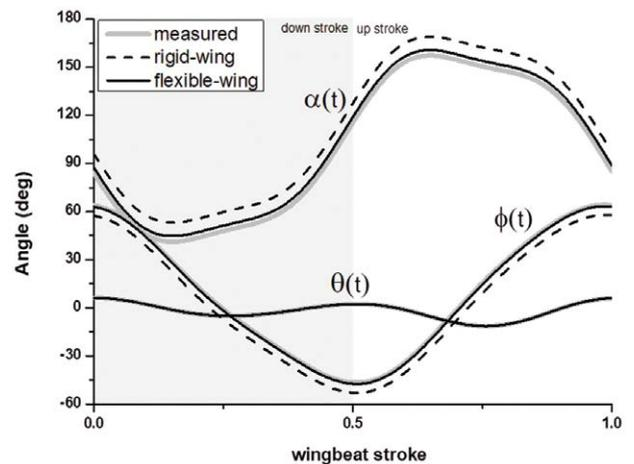
Figure 5. Flight kinematic inputs for the hovering condition
