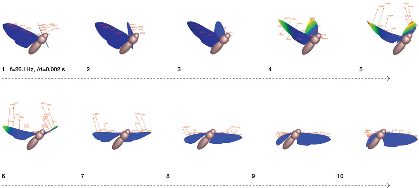
**Figure 6. Fluid-structure interaction considered 6-DOF free flight simulation; flexible-winged Hawkmoth model is in its hovering condition; a down-stroke wing motion is depicted (flapping frequency = 26.1Hz, time between each frame is 2ms)**
