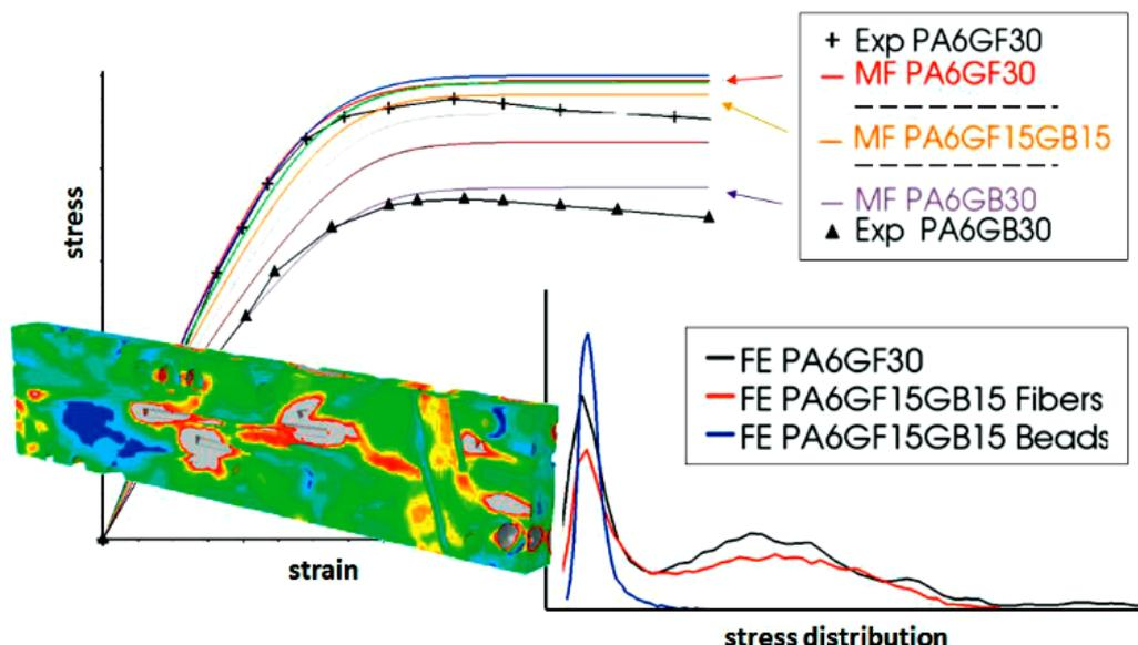
Figure 4 : In-depth investigation of new material compounding
