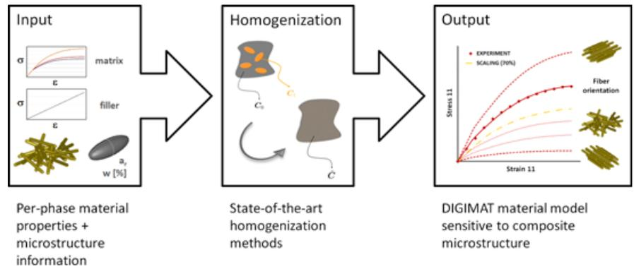
Figure 1: Homogenization workflow in simulation software (Digimat)
