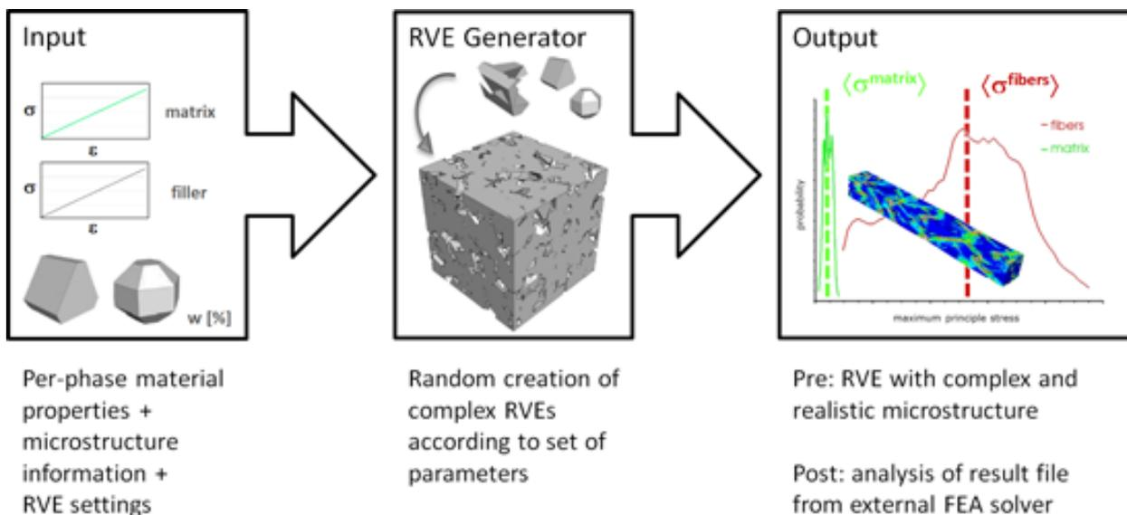
Figure 3 : Finite element-based homogenization workflow
