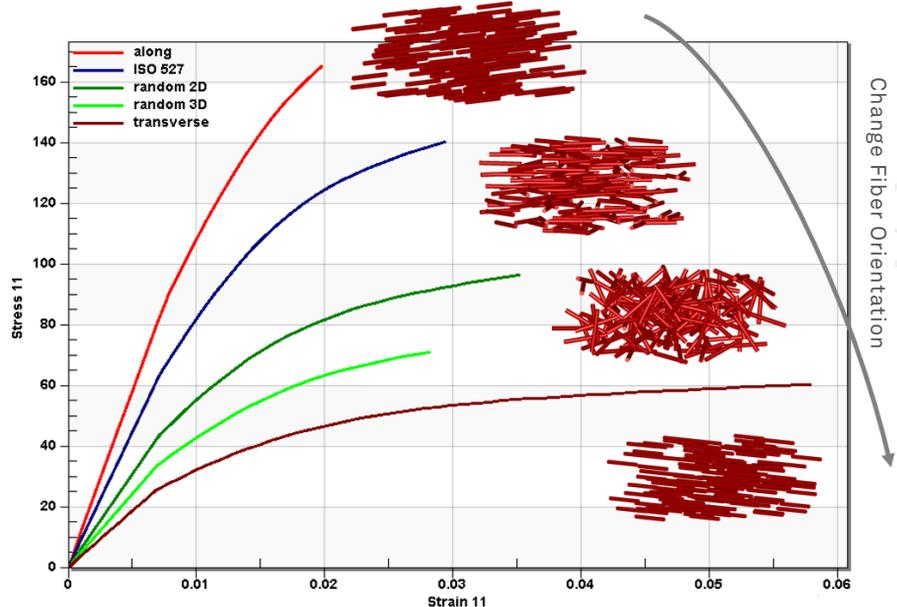
Figure 2: Influence of fiber orientation on SFRP non-linear behavior obtained by mean-field homogenization
