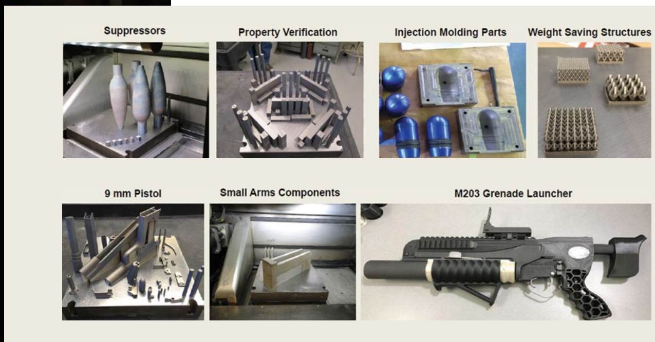
Figure 2: Metals AM Build Examples for the US Army at CCDC Armaments Center
