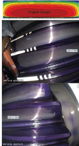
The more complex Romax model with FE housing (top), contact pattern after refinement matching the test rig results (top right), contact pattern after further optimisation (bottom)
