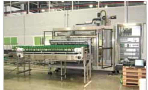
High-speed infeed machine for bottles: physical prototype
